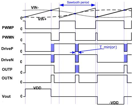
Figure 2- MP1720 operation diagram (with input signal) (not to scale)
