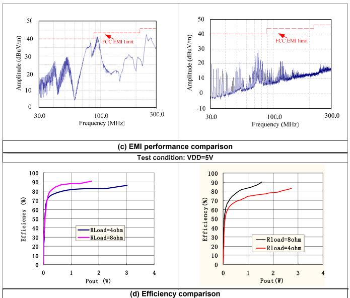
Figure 6, the different slew rate and corresponding performances comparison
