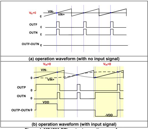
Figure 4, MP1720 BTL output operation waveform
