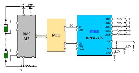
Figure 6: MPF42790 Typical Application Circuit
