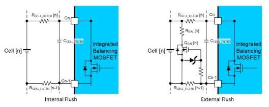
Figure 3: Cell Balancing Reference Circuit
