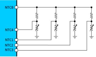
Figure 2: Four-Channel NTC Sampling
