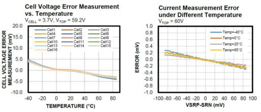
Figure 1: Cell Voltage Measurement and Current Measurement Error Curves
