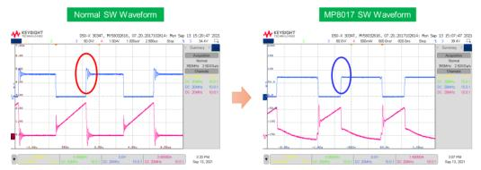
Figure 8: MP8017's Smooth SW Waveforms Attenuates EMI Sources
