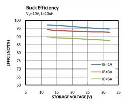
Figure 3: MP5515 Buck Efficiency Curve (V<sub>B</sub> = 10V)
