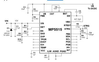
Figure 4: MP5515 Typical Application Circuit and Required External Components
