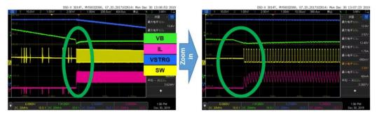
Figure 8: MP5515 Shutdown Transition Waveforms
