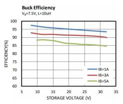
Figure 2: MP5515 Buck Efficiency Curve ( $V_B = 7.5V$ )
