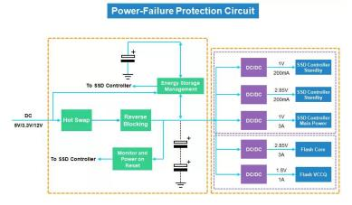
**Figure 11: Power Failure Protection Circuit**
