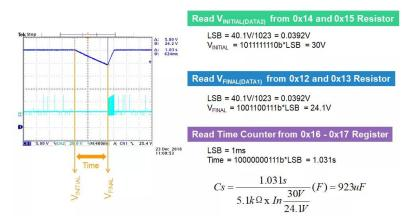
Figure 6: MP5515 Energy Storage Capacitor Detection Circuit Power
