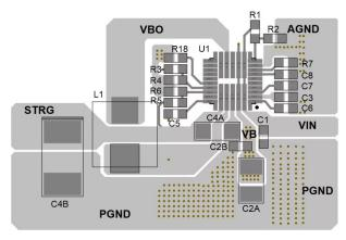
Figure 5: MP5515 PCB Layout
