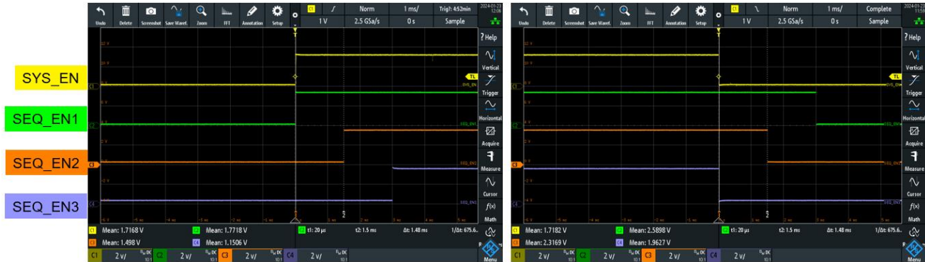
Figure 2: Start-Up and Shutdown Sequences of Tree Groups for Intel Agilex
