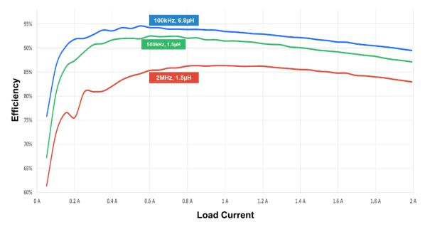
Figure 2: Efficiency Curves at Different Frequencies
