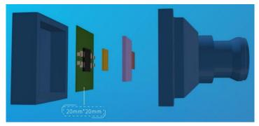
Figure 4: Onboard Camera Sensor
