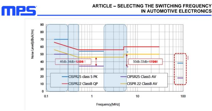
Figure 3: CISPR25 Class 3 CE Limit Standard Chart
