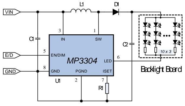
Figure 1—Application for Driving WLED Array
