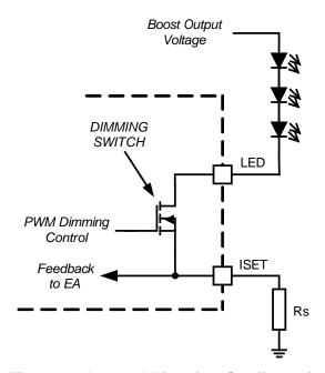
Figure 3—Internal Dimming Configuration
