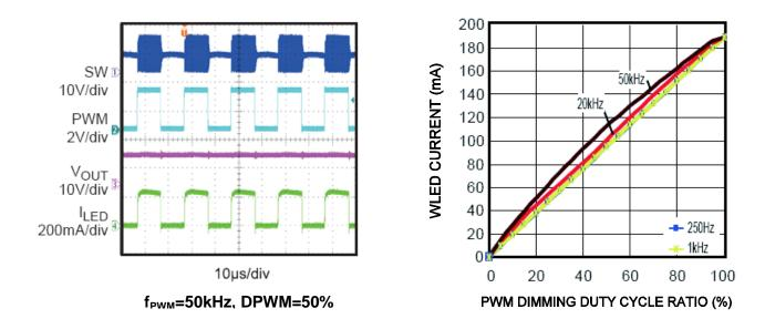
Figure 4—The Dimming-test Waveform and Curve for Reference Design
