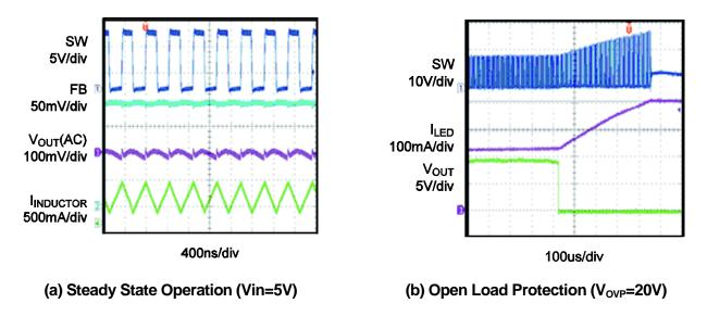
Figure 2—The Bench-test Waveform for Reference Design
