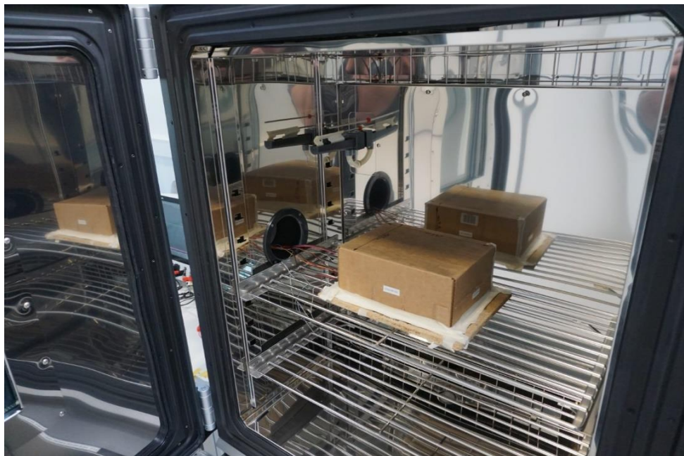
Figure 6: DUT PCB Under a Closed Carton in the Climate Chamber
