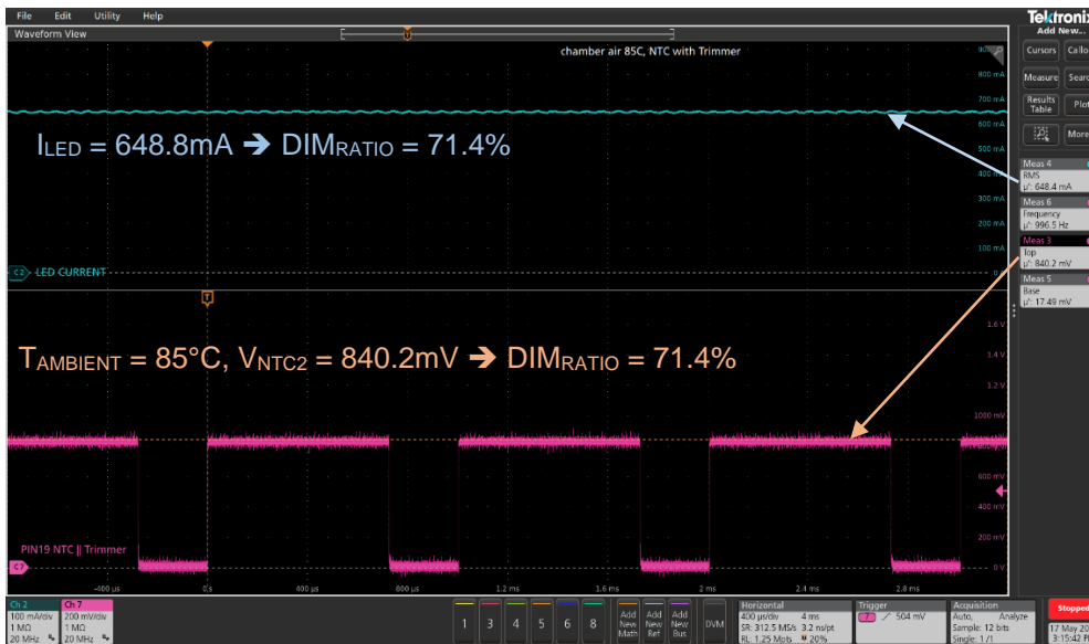
Figure 12: Measured V_{NTC2} at the NTC Pin ( V_{NTC2} = 840.2mV , I_{LED} = 648.4mA , T_{AMBIENT} = 85^\circ C )
