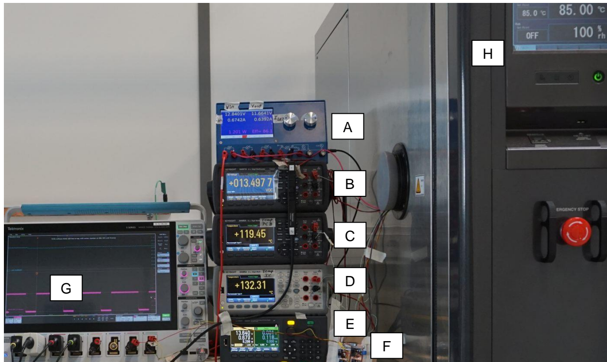
Figure 3: MPQ7200 Measurement Set-Up for NTC Thermal Dimming Derating
