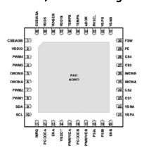
**QFN-40** (6mmx6mm), 0.5mm Pitch
