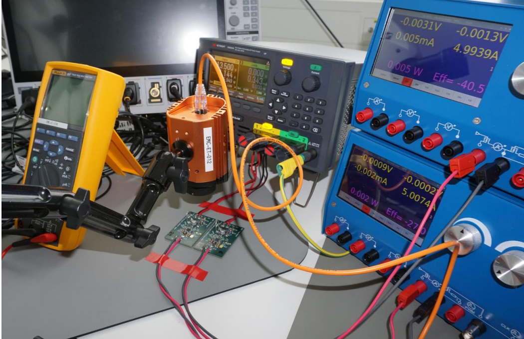
Figure 5: Test Set-Up for Efficiency and Infrared Thermal Images
