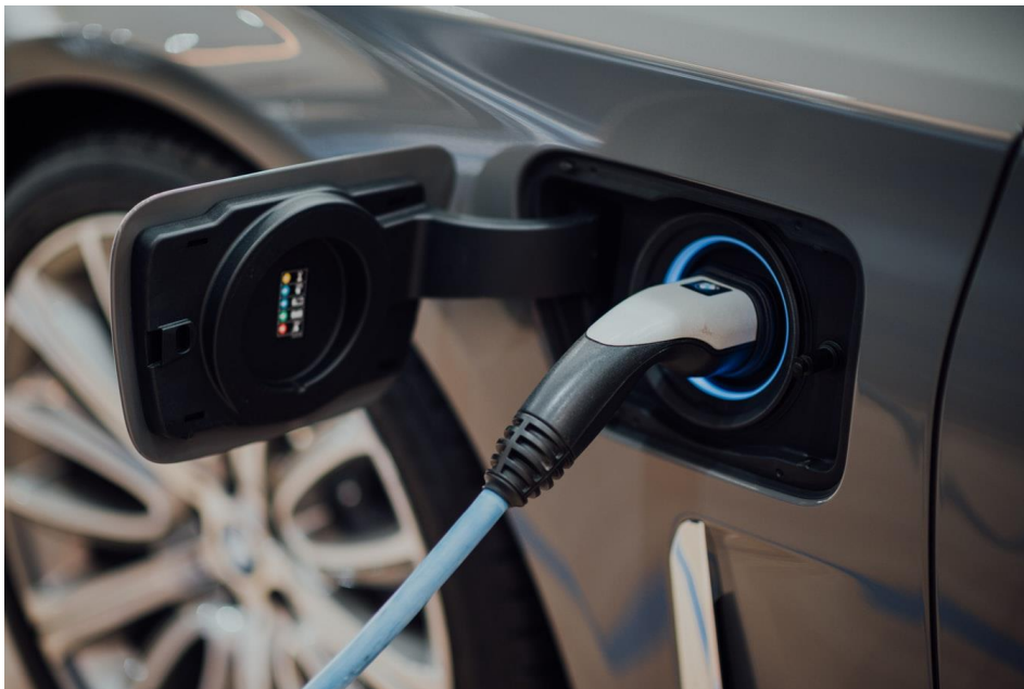
Figure 1: Electric Vehicle Being Plugged into an AC Charger
