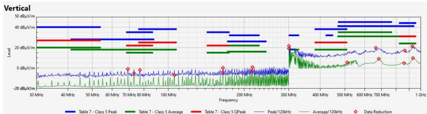
VERTICAL: No modifications, with 15cm cables
