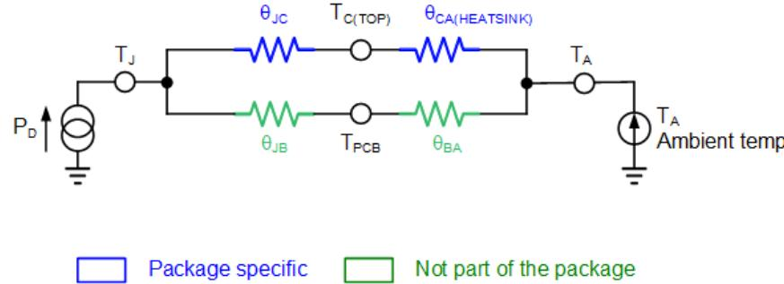
$\theta_{JB}$ : Thermal impedance from the die to the board.  $\theta_{JB}$  includes some of the board characteristics and their coupling with the package.
