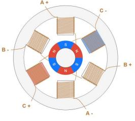
Figure 1: Stepper Motor
