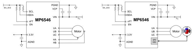
Figure 6: Input Mode (Left: Hall Sensor, Right: Magnetic Angle Sensor)
