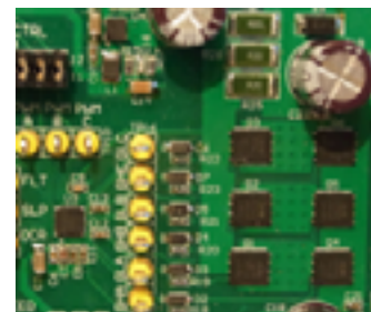
Pre-Driver plus 6 MOSFETs: 50mmx30mm
