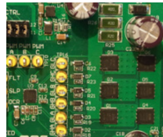
Pre-Driver plus 6 MOSFETs: 50mmx30mm
