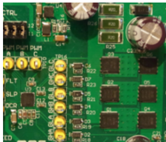
Pre-Driver plus 6 MOSFETs: 50mmx30mm
