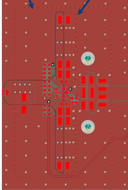
The diagram shows a PCB layout similar to TB6. A dashed red line indicates a split in the top-layer ground plane. A blue arrow points to the top-layer cut. The internal layer ground is shown as a solid, unsplit plane.
