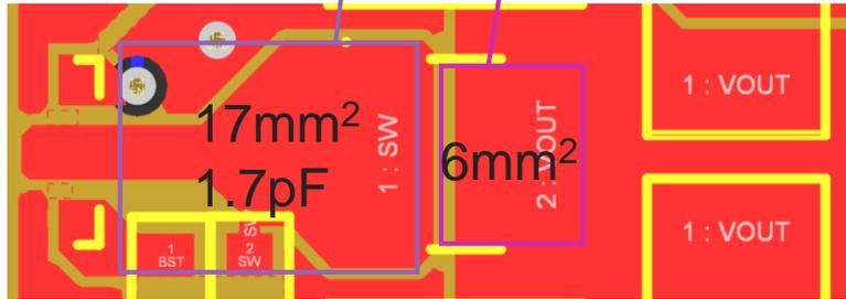
The copper area under the inductor in the top layer is  $V_{OUT}$ . The eddy currents are induced there. The parasitic capacitance between SW and  $V_{OUT}$  is increased by this additional area.
