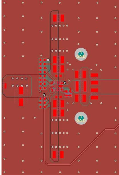
The diagram shows a PCB layout similar to TB6. The top-layer ground plane is solid and unsplit. The internal layer ground is also solid and unsplit.
