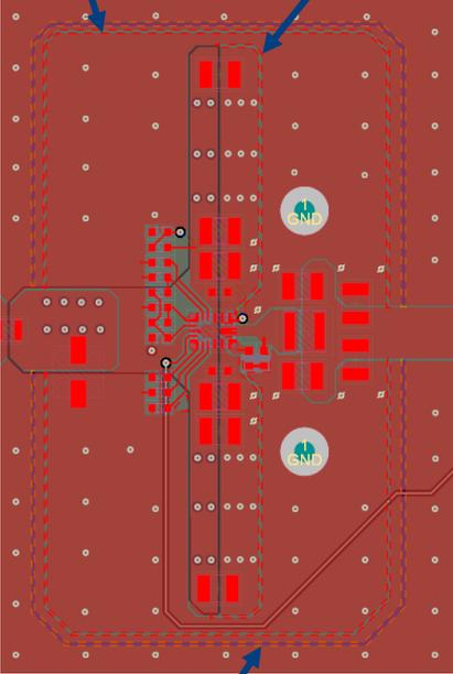
The diagram shows a PCB layout with a central component area. A dashed red line indicates a split in the top-layer ground plane around the component. A blue arrow points to a cut in the ground plane on the internal layer, also following the component's outline.
