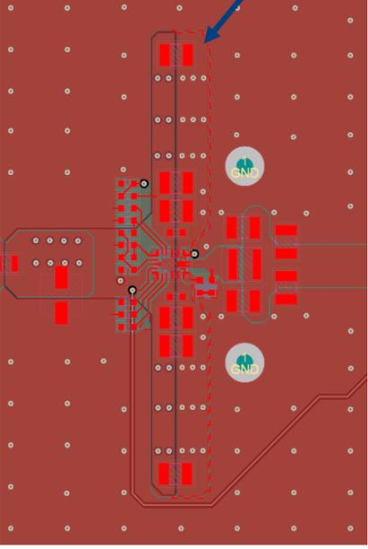
The diagram shows a PCB layout similar to TB6. A blue arrow points to a cut in the ground plane on the internal layer. The top-layer ground plane is solid and unsplit.
