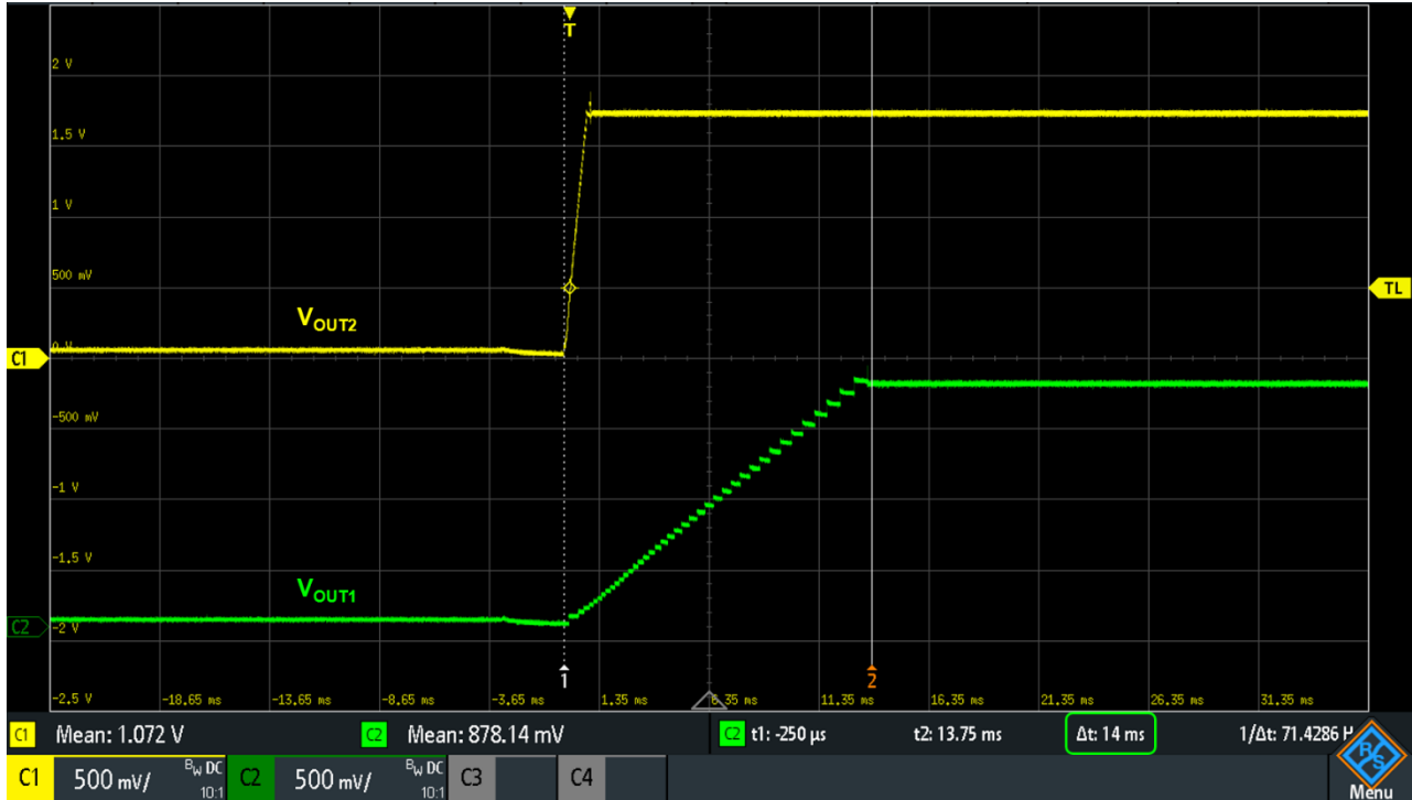
Figure 2: Start-Up Sequence with Two Independent Rails
