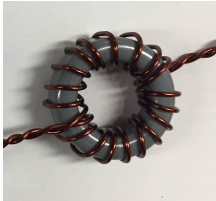
CM Inductor w/ DM current excitation
