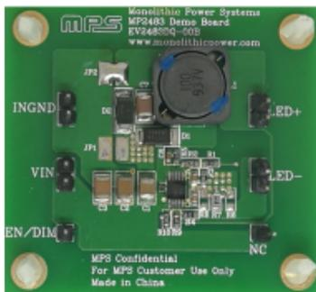
$V_{SW}$ ,  $I_D$ ,  $Z_{GND1}$ ,  $Z_{GND2}$  are most important for radiated EMI on this Board
