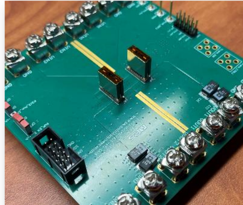
MPS' VRM solution in dual phase demonstration
