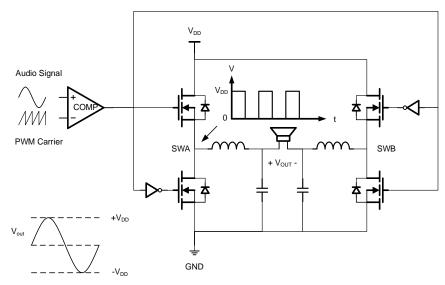
Figure 3: MPQ7795-AEC1 BTL Class-D Amplifier
