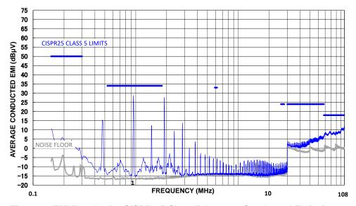
Figure 7: EMI Results for CISPR 25 Class 5 Average Conducted Emissions
