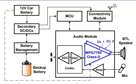
Figure 2: E-Call System (Simplified Block Diagram)
