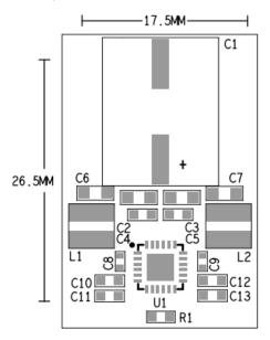
Figure 5: Small PCB Area of the MPQ7795-AEC1
