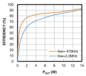
Figure 4: MPQ7795-AEC1 Efficiency Curve
