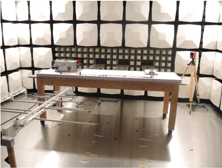
Radiated EMI measured with antenna
