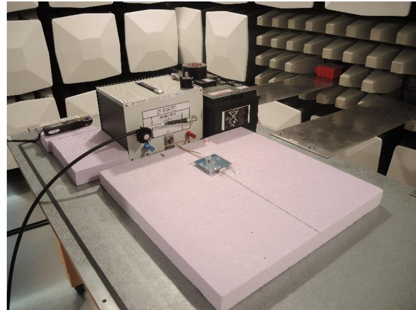
Conducted EMI measured through the cable with a LISN*
