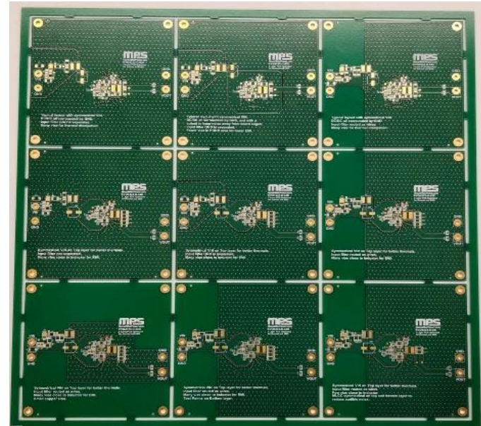
PCB Panel with 9 Different Layouts
